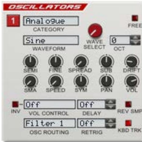
An oscillator is a tone generator. It is the first building block in the sound construction process. The frequency setting of the oscillator determines the pitch of the sound. The selected waveform defines the sound's initial tonal character, or timbre. Vecto uses 4 oscillators per voice (note played).
