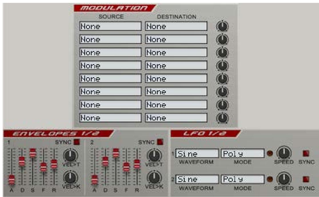
You find Vecto's modulation section in the bottom left hand corner of the panel. The modulation section holds 2 Envelopes, 2 LFOs and a modulation matrix with 8 slots. The modulation section is a treasure trove for subtle or complex sound-shaping options.
