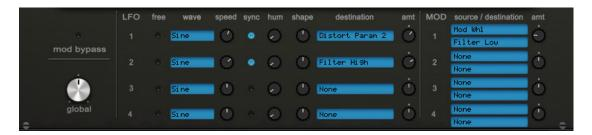
The modulation section gives you the opportunity to change RP DISTORT-RE parameters dynamically. For this purpose there are 4 independent LFOs and 4 freely configurable modulation slots at your disposal. There are two controls that affect all modulators simultaneously:
