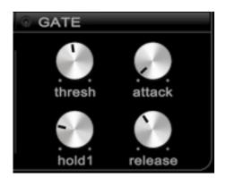
The noise-gate is an audio effect that removes any signal ('gates') that is below a threshold volume. It is typically used to keep noisy effects under control when no or a very low input signal is present. Distortion effects work with potentially very high internal amplification levels, which may lead to higher noise levels in the output stage.
