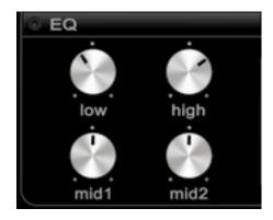
The EQ Unit is a four (4) Band Equalizer. The frequency bands are fixed at 125 Hz, 500 Hz, 2 kHz and 8 kHz. Each frequency band can be boosted or attenuated independently.
