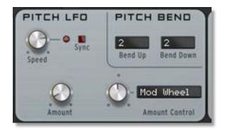
The Pitch section gives you control over the overall pitch of the sound. Think of using an LFO to generate vibrato or bending notes with the pitch bend controller.
