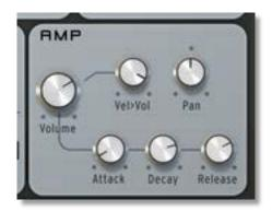
While the guitar model determines the basic sound and the filter section the timbre, the amplifier section is responsible for the sound's volume and panning. It amplifies the signal and modifies the volume. An important component of the amplifier section is the Volume Envelope. The envelope defines the loudness contour. The amplifier section also contains the velocity control. This sets the response of RG-RE to the velocity information.
