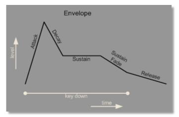
To hear the full effect of the Filter Envelope you have to open the Env amount, which you can find in the filter section next to the Cutoff Frequency. The amount can be positive or negative.
