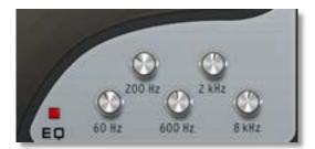
RG-RE includes a 5-band equalizer to further shape the sound. The LED-Style button turns the equalizer On and Off. The equalizer uses 5 bands at the following frequencies:
