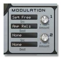
The modulation slots define modulation paths where a source is assigned to change a destination parameter. Internal modules such as envelopes and LFOs, and external MIDI controllers such as pitch bend, aftertouch and other control messages defined in the midistandard may be used a source. Possible modulation targets are a large set of RG-RE's internal parameters. A full list is provided at the back of this manual.
