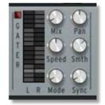
The gater uses a 16 step sequencer to alter the volume of the sound to give a trance-gate type effect. Basically it is a sequencer controlled audio gate.
