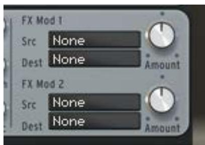
The FX modulation slots work similar to the generic Matrix modulation slots. The difference is that as modulation destinations, you can only choose from effect parameters as specified in the effects type section. A full list is provided at the back of this manual.
